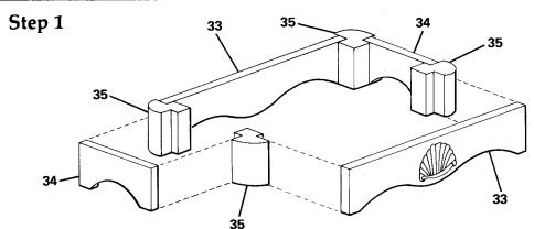
A. Assemble frame by gluing side aprons (33) and end aprons (34) into notches of corners (35). Top edges of all parts should be flush. Square assembly and allow glue to set.
