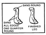
NOTE: Legs may be shaped prior to assembly sanding as shown.
